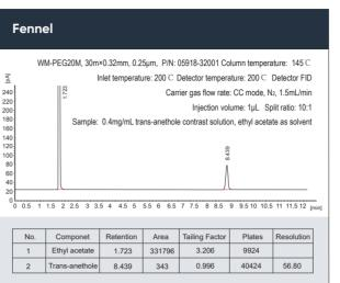
Inlet temperature: 200 °C Detector temperature: 220 °C Detector FID
