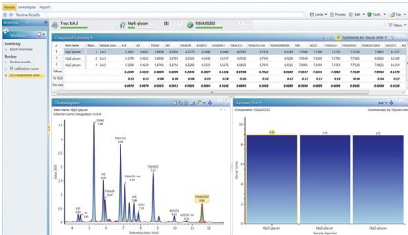
Figure 4. A component summary table in the review page that compares the GU value for all the identified glycans across a triplicate injection of a glycan mixture sample. Summary calculations for individual glycans across triplicate analysis of the glycan test standard are presented in the component summary table.
