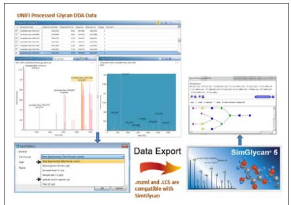
Figure 3. Workflow 2: Glycan DDA workflow in UNIFI Software. Collision-induced dissociation (CID) of glycans in data dependent acquisition (DDA) mode is processed and exported to SimGlycan.
