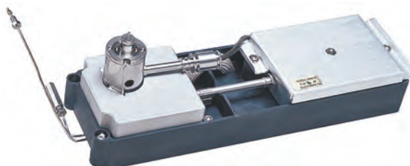
D-3-I-HP PLUG-IN SYSTEM for Agilent 6890 GC
