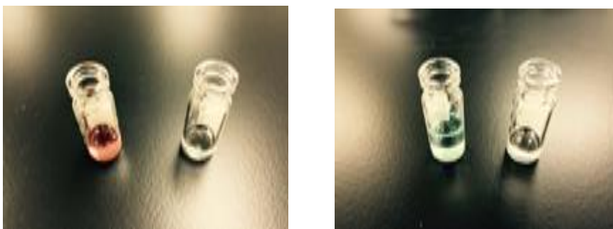
Figure 4: Comparison of QuEChERS extracts before and after dSPE cleanup (from left to right: hard candies and gummies)
