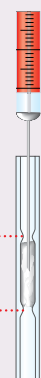
Figure 2 The two tapered sections secure the quartz wool plug effectively wiping the needle tip during injection. This results in improved reproducibility.
