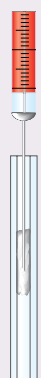
Figure 3a Quartz wool plug is in the position to wipe needle tip.
