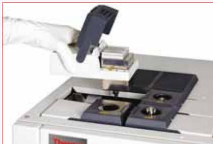
Example of instant connect module installation by user
