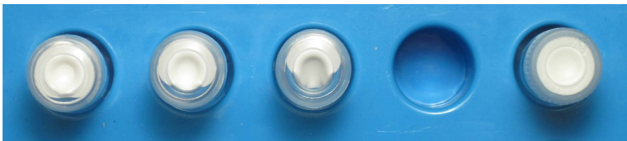
Figure 4. Septum displacement due to overtightening of the closure compared to SureStop vial under excessive torque.
