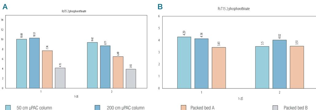
**Figure 7. Resolution obtained between diastereomers of T5 and T15 oligonucleotides with 2 phosphorothioate linkages, respectively on the left (A) and right (B).** 50 cm and 200 cm μPAC columns have been compared to two silica based C18 packed bed columns (packed bed A and packed bed B). Flow rate 250 nL/min, 30 min gradient 20 to 70% B, A: 100% H<sub>2</sub>O, B: 40% acetonitrile with 15mM TEAA in both A-B, UV 260 nm.
