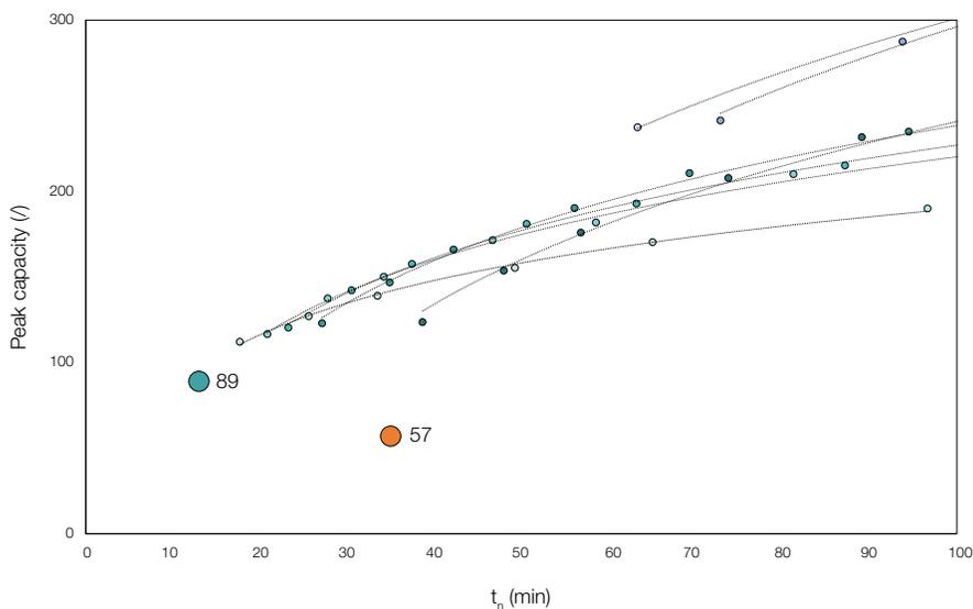
**Figure 10. FWHM based peak capacity obtained for a 5mer deoxythymidine oligonucleotide with 4 phosphorothioate linkages (T5-1-4S) on either a 50 cm  $\mu$ PAC column and 15 cm packed bed A column.** Peak capacity within the diastereomer elution window is calculated based on the peak width of a baseline separated peak and plotted as a function of  $t_n$ , retention time of the last eluting oligonucleotide diastereomer. Data points have been obtained from separations shown in Figure 9.
