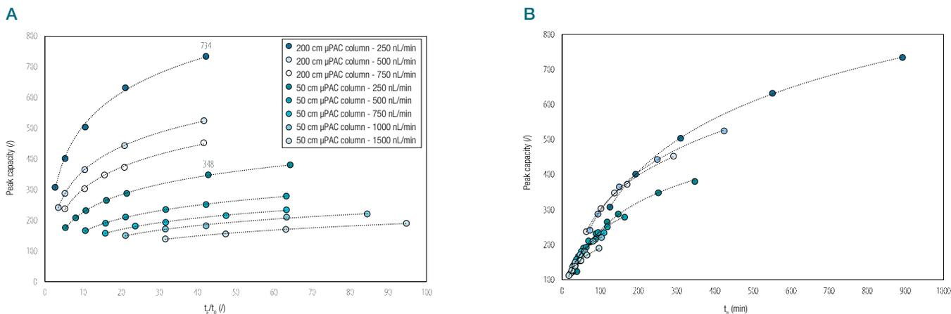
**Figure 3. FWHM based peak capacity obtained for an oligonucleotide reference standard mixture (T5-T30).** The performance obtained on a 200 cm and a 50 cm μPAC column is compared at different flow rates (250–1500 nL/min). A) Peak capacity plotted as a function of  $t_E/t_0$ .  $t_E = t_n - t_1$ . B) Peak capacity plotted as a function of  $t_n$ , retention time of the last eluting oligonucleotide (T30).
