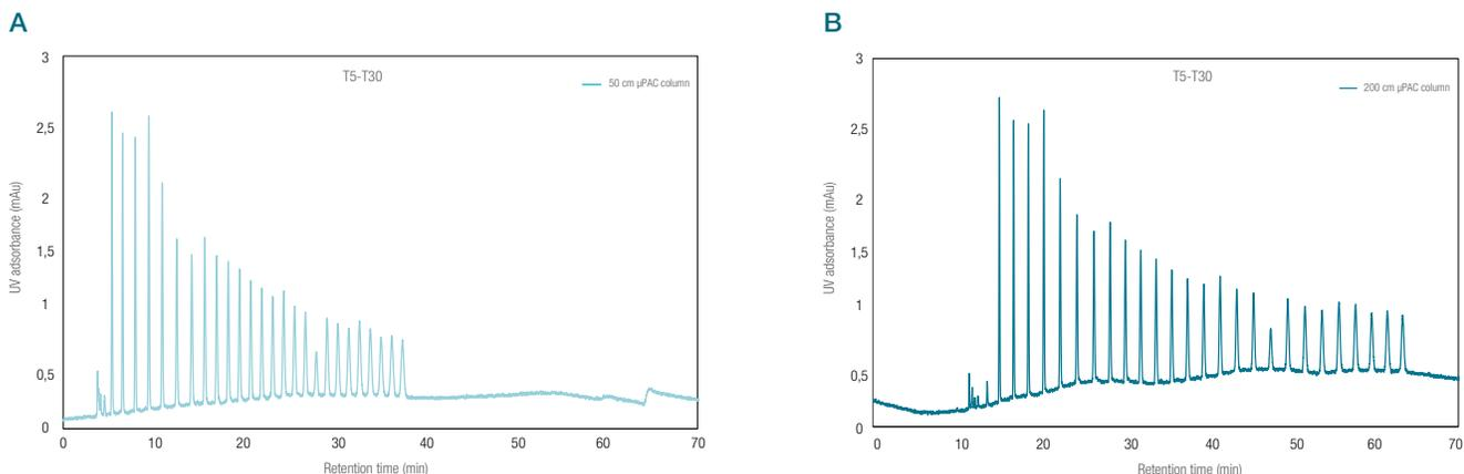
**Figure 2. UV chromatograms obtained for the separation of 5-30mer deoxythymidines (dT<sub>s</sub>) on either A) the 50 cm μPAC column or B) 200 cm μPAC column.** Flow rate 750 nL/min, 60 min gradient 20 to 70%B\_C2 curve, A: 100% H<sub>2</sub>O, B: 40% MeOH, UV 260 nm.
