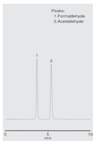
Chromatogram of Standard Sample (formaldehyde 0.35 μg/mL, acetaldehyde 0.55 μg/mL, 10 μL injected)
