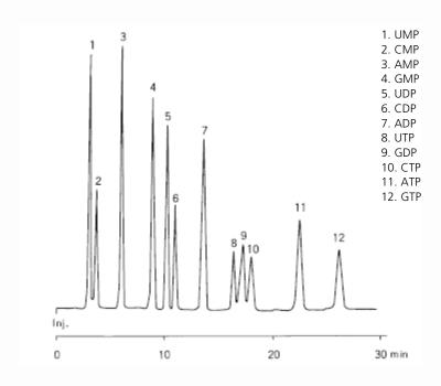
Column : Shim-pack WAX-1 (50 mm x 4.0 mm I.D., 3 μm), P/N : 228-16225-91
