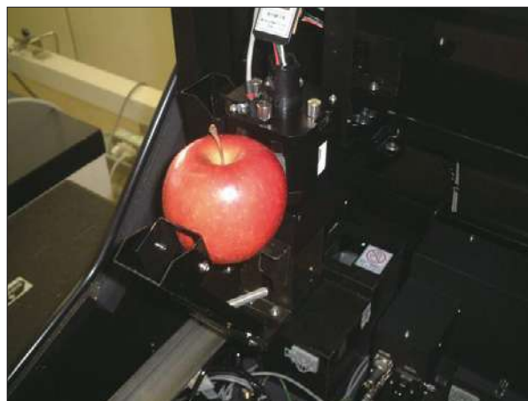
Fig. 1 Apple Mounted in Integrating Sphere
