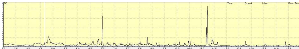
Figure 8B: Total Ion Chromatogram of Pears QuEChERS Extract (scan mode)
