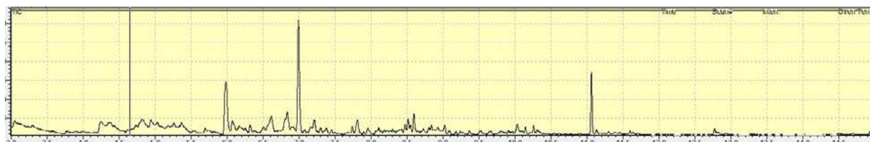
Figure 8D: Total Ion Chromatogram of Peas QuEChERS Extract (scan mode)
