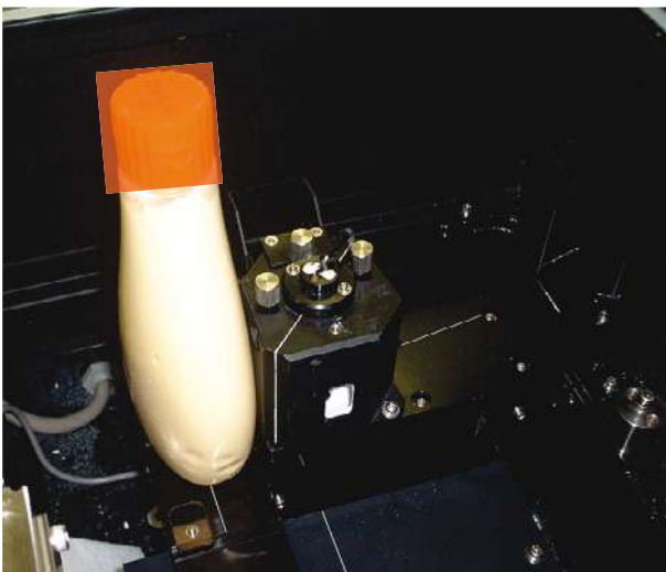
Fig. 5 Sample Set in an Integrating Sphere
