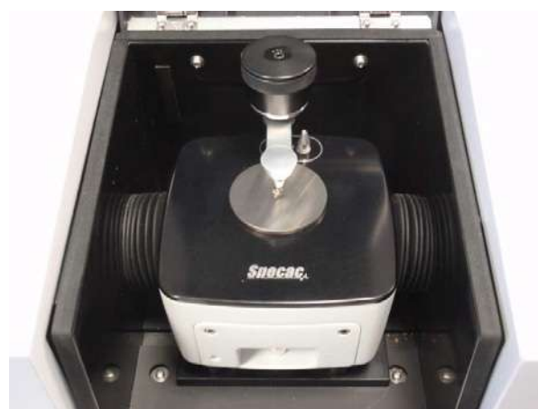
Fig. 2: Single reflection ATR – The Quest, a full diamond ATR version from Specac, mounted to Shimadzu FTIR sample compartment
