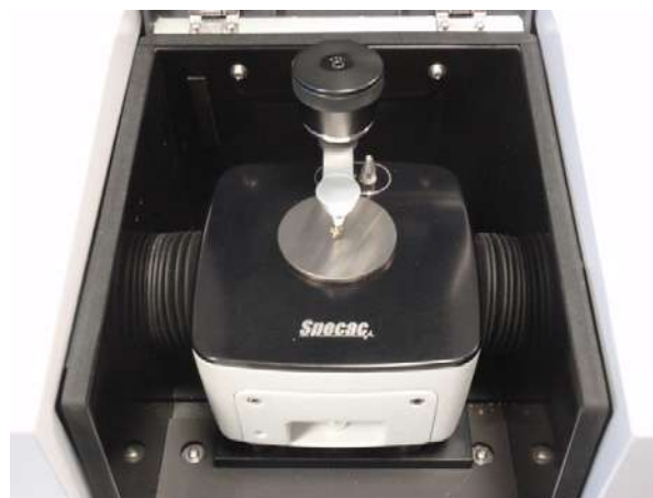
Fig. 4: Single reflection ATR – The Quest, a full diamond ATR version from Specac, here shown as part of an IRAffinity-1 from Shimadzu
