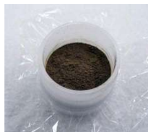
Fig. 3 Seaweed Hand-Pressed (Easy Press) into Cup
