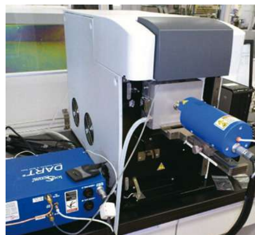
Fig. 2 DART-SVP Ion Source Coupled with LCMS-2020 Single Quadrupole Mass Spectrometer
