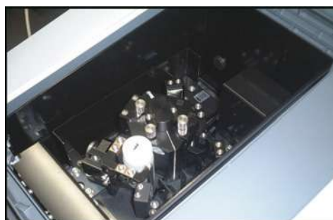
Fig. 2 Sample Set in Integrating Sphere Attachment
