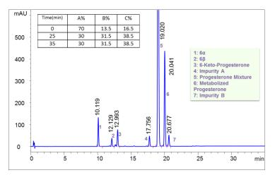
Opalshell<sup>™</sup>-C18 (2.6 μm, 90 Å, 4.6 x 50 mm) Column: Mobile Phase: A :H<sub>2</sub>O; B: ACN; C: MeOH (v/v)Injection: 10 µL Flow Rate: 1.0 mL/min Pressure: 120 bar Detection: UV 241 nm Temperature: Ambient Sample: Progesterone sample mixture (0.5 mg/mL)
