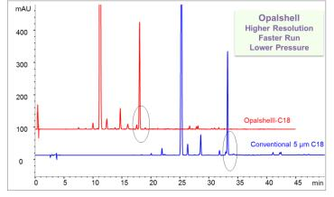
Column: Opalshell<sup>™</sup>-C18 (2.6 µm, 4.6 x 50 mm) C18 ( 5 µm, 4.6 x 250 mm) Mobile Phase: A: 0.1% Acetic Acid in Water, B: ACN Injection: 20 µL Flow Rate: 1.0 mL/min Pressure: 105-165 bar Detection: UV 254 nm Ambient Temperature: Prednisolone Acetate Tablets (0.05mg/mL) Sample:
