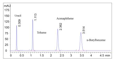
Column: Mobile Phase: Injection: Flow Rate: Detection: Temperature: Sample: Opalshell<sup>™</sup>-C18 (2.6 μm, 4.6 x 50 mm) ACN : H<sub>2</sub>O = 60 : 40 (v/v) 1 μL 1.5 mL/min UV 254 nm Ambient Uracil (0.05 mg/mL) Toluene (5 μL/mL) Acenaphthene (1.2 mg/mL) n-Butylbenzene (10 μL/mL)
