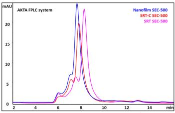
SRT SEC-500 best separated the aggregates of Ferritin in the presence of detergent.
