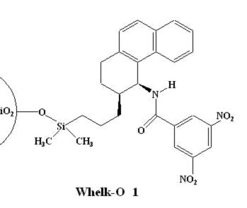
Since the phase is covalently bonded to silica, the column is compatible with all commonly used mobile phases and can be used for both normal phase and reversed-phase separations.
