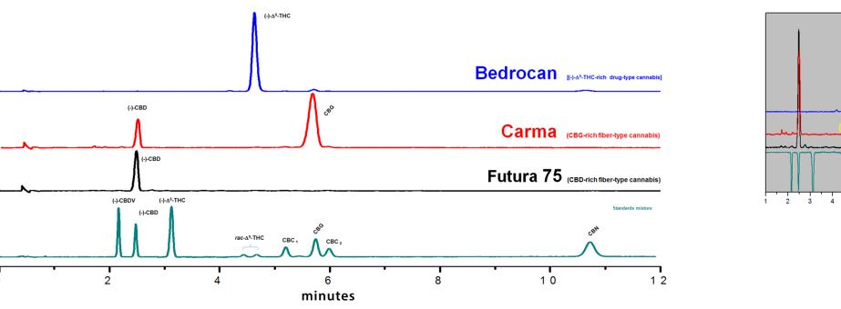
Standard Mix: 0.17 mg/ml Eluents : A) CO<sub>2</sub> B) MeOH 98:2 Isocratic condition: 98:2; Flow: 3.5 mL/min; DPi: 4260 PSI; ABPR: 1500 PSI Pumps: UPC<sup>2</sup> Waters Cell: 8 ml; UV @ 214 nm; T<sub>col</sub>: 30°C; V<sub>ini</sub>: 1 μl
