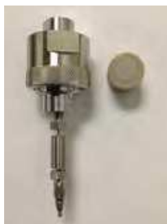
Holder for 4.0 and 2.0 mm i.d. cartridges
