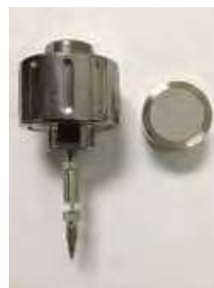
Holder for 21.2 mm i.d. cartridges
