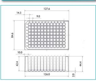
A new introduction to the Porvair range is a low profile 1.2ml 96-well round plate with a height of just 27mm. This allows more plates to be stored or stacked in a given space. The plates are made with extractable-free polypropylene for excellent results. A specific anti-evaporation cap mat is also available for this plate manufactured from thermoplastic elastomer.
