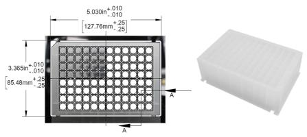
Porvair Sciences 96 deep well plate is designed to tight specifications required for full compatibility with all Thermo Scientific™ KingFisher™ automated purification systems.
