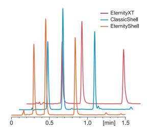
In this separation of steroids, the same analysis is carried out on three C18 columns from different Kromasil families.
