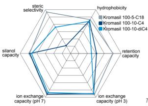
Kromasil® diC4 has strong C4 characteristics in terms of capacity and hydrophobicity. The main difference is a steric selectivity in between a C18 and a C4, more like a C8.
