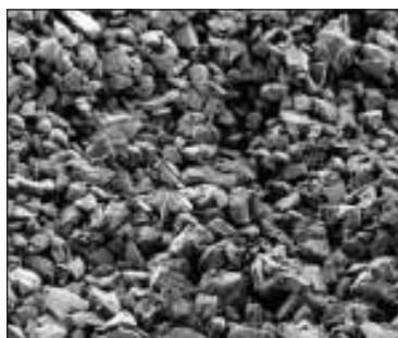
(A) classical silica TLC plate
