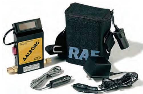
Left: Flowmeter; Right: Battery kit with battery pack (back right), battery to flowmeter cable (front center), and battery AC power cord (front right)
