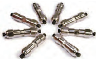
Photograph of the 8-column SMB set. Each perfectly-matched column is 5 cm x 10 mm I.D.
