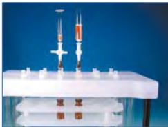
4. The shelves are then secured on the rack posts by attaching the "C" shaped support clips to the slots in the support posts directly under the shelf that is to be supported.
