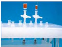
2. Just before you do your final elution, remove the lid, and take the waste tank containing the waste solvents out of the glass vacuum chamber. There are small handles at each end of the waste tank to facilitate its removal.
