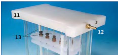
Figure 4: Vacuum manifold with drying attachment
