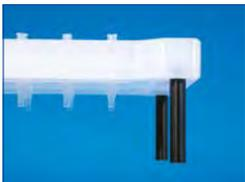
2. Check to ensure that the white plastic lid gasket is properly seated in the lid.
