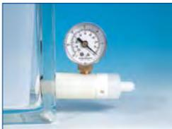
Do not allow vacuum to go below 20 inches of mercury (68 kPa, 680 mbar, 510 Torr, 0.66 atm, 0.67 bar, 9.8 psi). Exceeding this vacuum will void the manifold warranty. For most applications a region of 25–27 inches of Hg (84–91 kPa) is satisfactory for proper flow through the CHROMABOND® SPE columns. The bleed valve ring also permits vacuum release for the purpose of changing collection vessels
