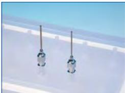
4. Insert the flow control valves (stop cocks) into the female luer fittings on the lid.
