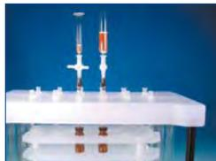
5. Waste solvents should be properly discarded from the waste tank. The tank can be rinsed and re-used a number of times before discarding. Using the waste tank will save time, and greatly simplify manifold clean-up following a sample run, by eliminating the necessity for cleaning the vacuum chamber between sample runs.
