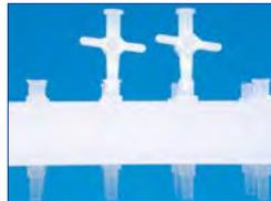
5. Rotate the valves slightly to ensure positive seating.
