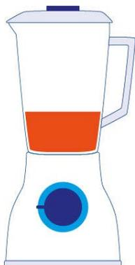
1. Sample is homogenized, e.g., with dry ice in a blender.
