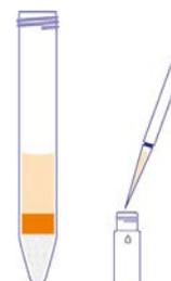
4. Transfer supernatant to vial, acidify with 5 % formic acid in acetonitrile (10  $\mu$ L/mL extract) and analyze sample by LC/MS or GC/MS.
