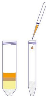
1. Transfer an aliquot of the supernatant to a centrifuge tube containing a clean-up mix. This dispersive solid phase extraction mix (dSPE) removes matrix components such as fats, sterols and pigments.
