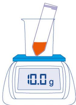
2. Weigh 10 g of the sample into a centrifuge tube.
