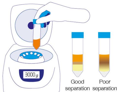
7. Centrifuge for 5 min at > 3000 g. For the determination of pesticides with acidic groups, the raw extract should be analyzed directly (preferably by LC/MS ESI neg.).
