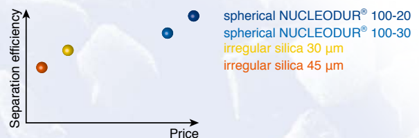
Comparison of separation efficiency and price of irregular versus spherical silica
