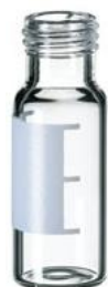
11 40 2556 HPLC/GC Certified Vial Kit: 1.5ml Short Thread Vial, 32 x 11.6mm, clear glass, 1 st hydrol. class, label; UltraClean Closure: 9mm PP Short Thread Cap, blue, centre hole; Silicone white/PTFE red, 55° shore A, 1.0mm
