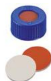
09 15 1819 9mm Combination Seal: PP Short Thread Cap, blue, with centre hole; RedRubber/PTFE beige, 45° shore A, 1.0mm
