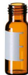
11 40 2557 HPLC/GC Certified Vial Kit: 1.5ml Short Thread Vial, 32 x 11.6mm, amber glass, 1 st hydrol. class, label; UltraClean Closure: 9mm PP Short Thread Cap, blue, centre hole; Silicone white/PTFE red, 55° shore A, 1.0mm
