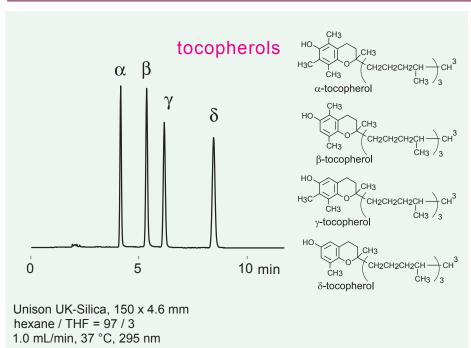
The Unison series of columns provides authoratative results in normal phase separation using its silica stationary phase. This high level of performance is in addition to its extraordinary resolution, higher than conventional 5um columns.
