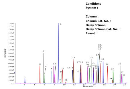
Exion HPLC System (SCIEX) QTRAP 6500+ LC-MS/MS System (SCIEX) InertSustain AQ-C18 ( $1.9 \mu m$ ,  $50 \times 2.1 mm$  I.D.) 5020-89938 Delay Column for PFAS ( $30 \times 3.0 mm$  I.D.) 5020-90005 A) CH<sub>3</sub>OH B) 20 mmol/L CH<sub>3</sub>COONH<sub>4</sub> in H<sub>2</sub>O
