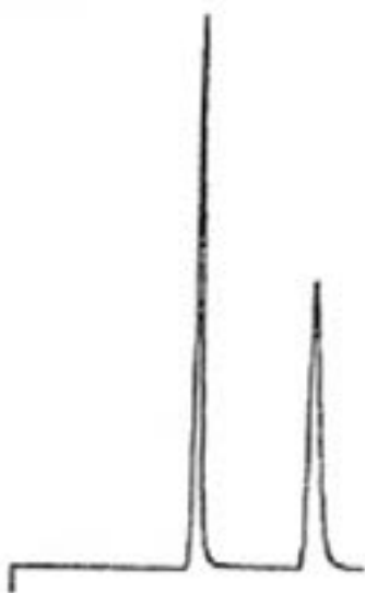
ChromegaChiral CCO F2 SFC Separation of Warfarin Mobile Phase: CO 2 :Methanol (80:20 v/v) Temperature: 10°C Flow Rate: 4 mL/min Pressure: 350 Bar
