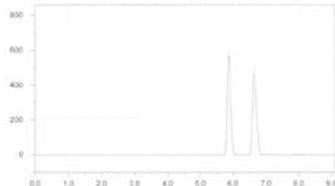
ChromegaChiral CCS Separation of 1-Indanol without DEA additive Mobile Phase: Hexane:IPA (90:10 v/v) Temperature: 25°C Flow Rate: 1 mL/min Detection: UV @ 254nm
