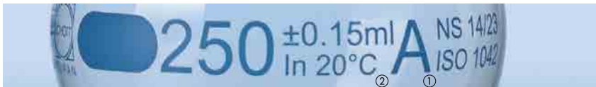
Tolerance indication with a volumetric flask in accuracy class A (①) with a tolerance of \pm 0.15 ml (②)
