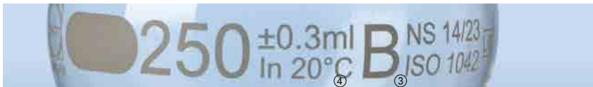
Tolerance indication with a volumetric flask in accuracy class B (③) with a tolerance of \pm 0.3 ml (④)
