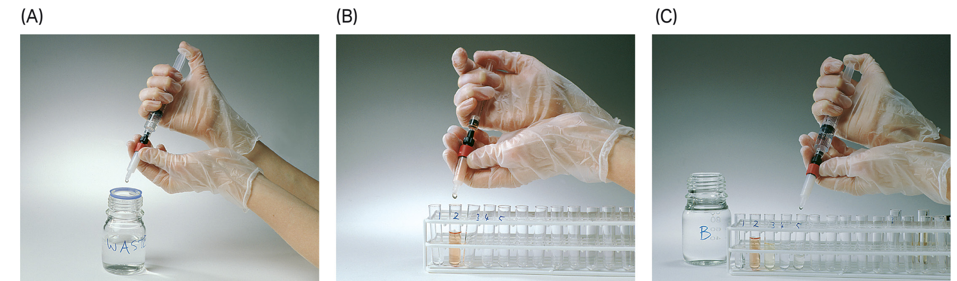
Fig 7.1. Using HiTrap columns with a syringe. (A) Prepare buffers and sample. Remove the column's top cap and twist off the end. (B) Equilibrate the column, load the sample, and begin collecting fractions. (C) Wash and elute, continuing to collect fractions. This procedure is particularly suitable for purification of tagged proteins, because a single step is expected to give a high degree of purification.
