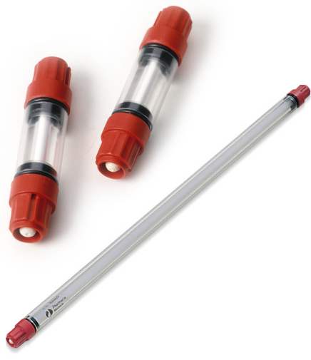
Fig 7.20. Precision columns. Examples: Mini Q PC 3.2/3 (at left); and Superdex Peptide 3.2/30 (at left).
