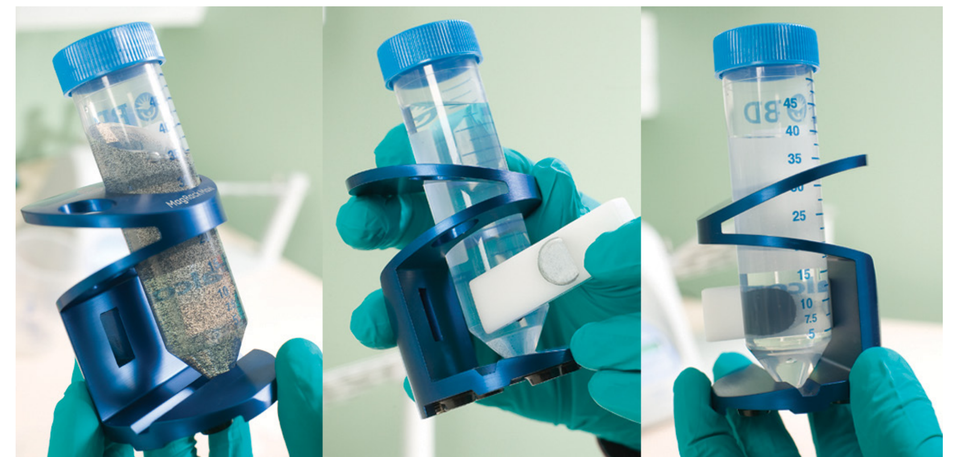
Fig 3.9. (A) MagRack 6 and (B) MagRack Maxi magnetic racks consist of an aluminum housing with a detachable magnetic bar. When the magnetic bar is inserted (center images), the high-density magnetic beads become attracted to the magnet in seconds. This allows easy removal of supernatant while the magnetic beads remain in the tube (images on the right).
