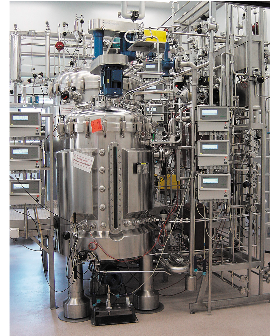
Fig 81A. 500 L stirred tank for microcarrier applications.
