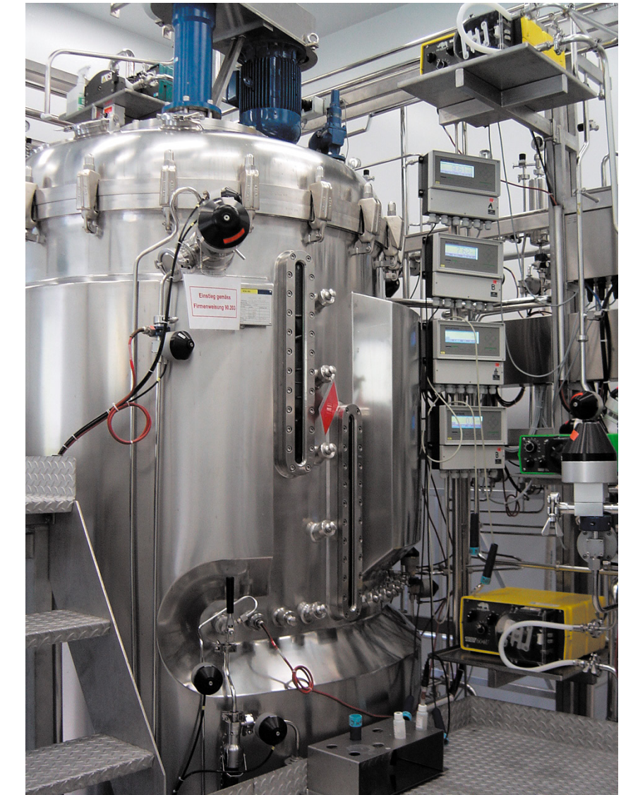
Fig 81B. 2000 L tank for microcarrier applications.
