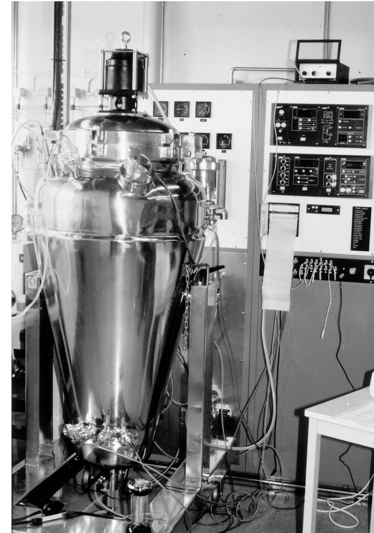
Fig 49. Example of a conically shaped stirred tank reactor.
