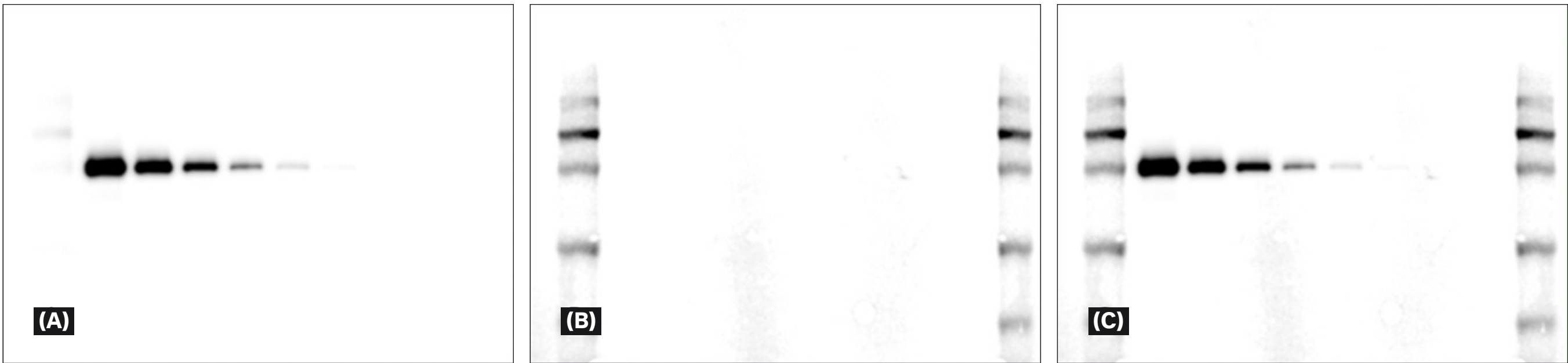
Fig 4.5. The three images of one chemiluminescent membrane showing (A) the chemiluminescent image, (B) the white light image of the colorimetric marker and (C) the overlay image in IQTL for display and analysis.
