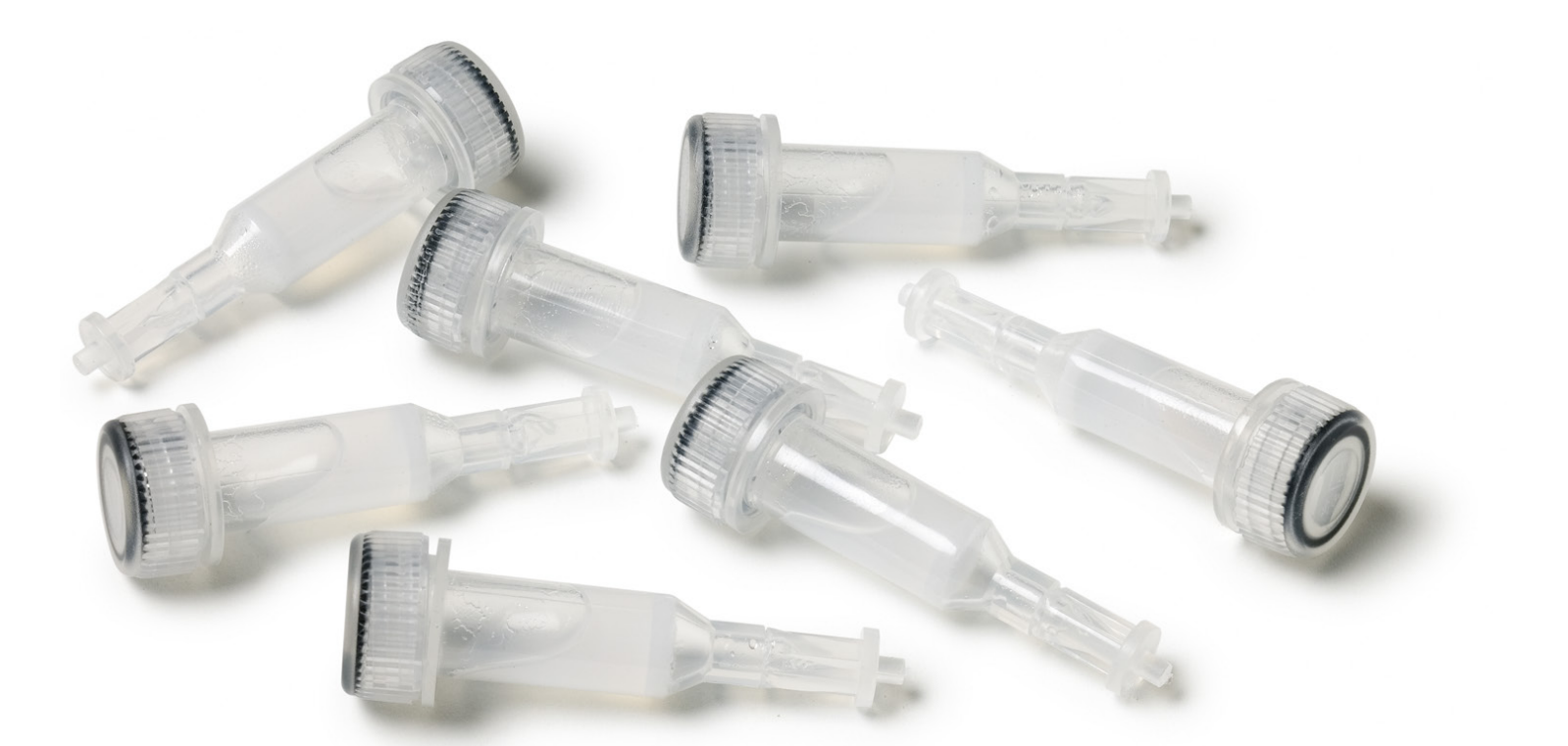
Fig 3.7. Protein G HP SpinTrap columns are used for protein enrichment of target proteins using antibodies bound to the protein G ligand and are also used for small-scale purification of antibodies.
