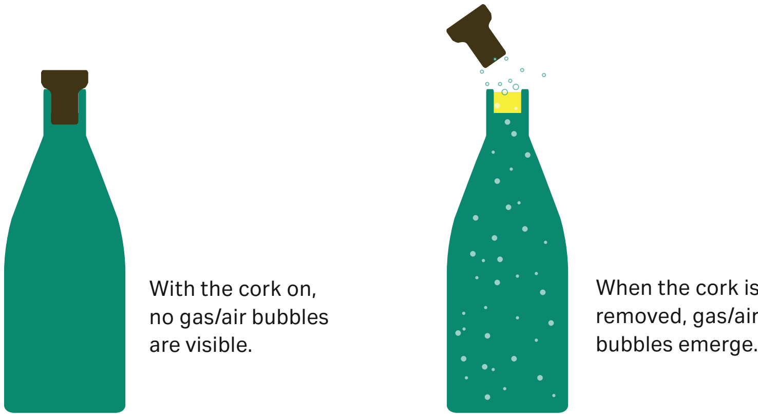
Fig 7.5. The flow restrictor can be compared to the cork on a champagne bottle.
