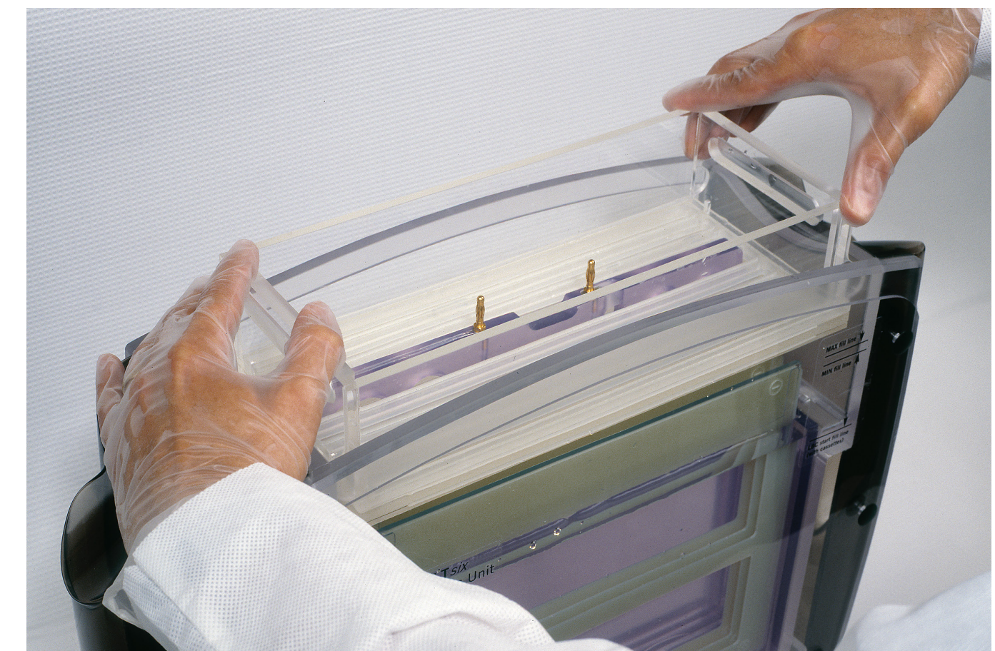
Fig 43. Seating the upper buffer chamber.
