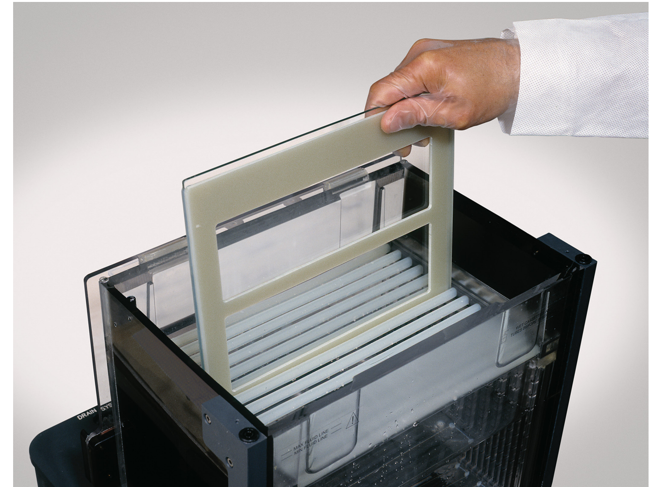
Fig 44. Loading the gel cassettes into Ettan DALTtwelve electrophoresis unit.
