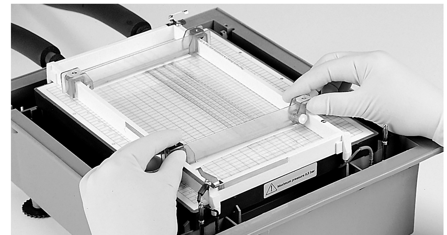
Fig 49. Alignment of electrodes over Immobiline DryStrip gels.
