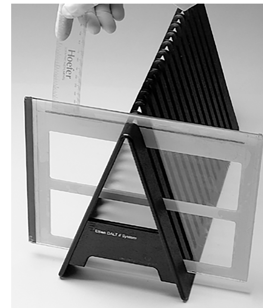
Fig 40. Pushing the Immobiline DryStrip gel down to contact the gel slab.
