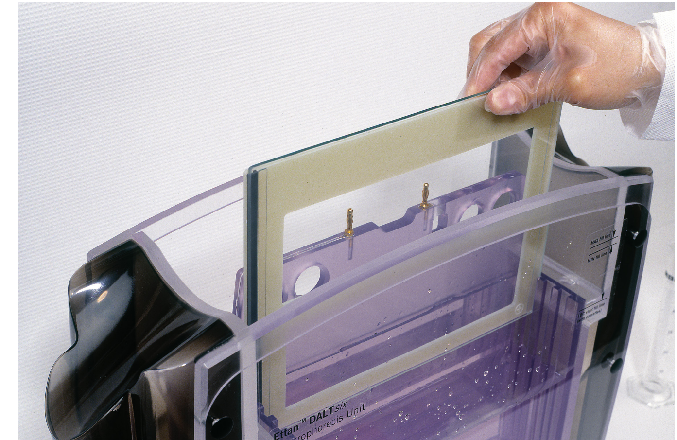
Fig 42. Inserting the cassettes into the cassette carrier.
