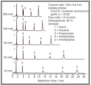
Separation on Sunrise C18-SAC is done including hydrogen bond and ion-exchange interaction based on silanol groups except for hydrophobic interaction. Control of pH and salt concentration of a mobile phase can regulate retention.
