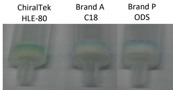
Figure(E). Comparison of column bed colour of three manufacturers' cartridges after loading same amount of Methyl Blue.
