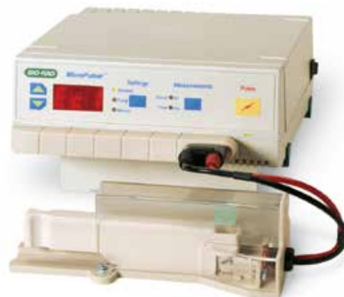
MicroPulser electroporator with cuvette chamber attached. Electroporator is shown connected to the cuvette chamber.
