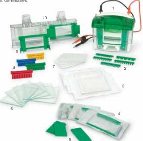
Mini Trans-Blot electrophoresis transfer cell components:
