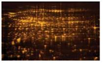
**2-D gel stained with Oriole stain.** *E. coli* protein (40 μg) was run on an 11 cm pH 5–8 ReadyStrip<sup>™</sup> IPG strip for the first dimension and a Tris-HCl 8–16% Criterion<sup>™</sup> gel for the second dimension.
