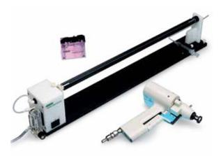
includes 15 m (50') of Tefzel tubing, five cartridge collection/ storage vials, five desiccant pellets, and 0.5 g of PVP for the sample tubing coating procedure. This is sufficient material (excluding nucleic acids, spermidine, CaCl<sub>2</sub>, and absolute ethanol) for preparing approximately 1,000 gene gun samples.
