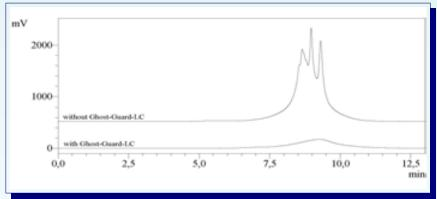
Analytical Platinum C18/C18 EPS; length: 33 mm, ID: 7 mm; Column  $1.5~\mu \mathrm{m}$ Mobile Phase A mixture of 950 ml water, 50 ml methanol and 0.1 ml acetone Mobile Phase B methanol Detection UV: 220nm Min % A % B 0 100 0 2 100 Gradient 7 10 90 8 100 0 13
