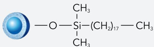
Built upon proven Fused-Core<sup>®</sup> particle technology for speed and efficiency, the HALO<sup>®</sup> OLIGO C18 incorporates surface modified organo-silane technology for alkaline resistance resulting in excellent stability under elevated pH operating conditions common in oligonucleotide separation methods.
