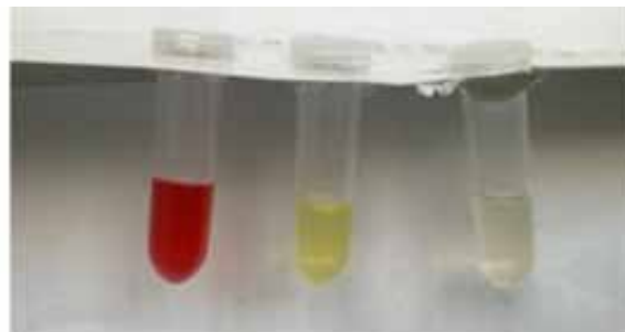
Cleanup of grape sample: Before cleanup (left), PSA (middle) and MWCNT (right)
